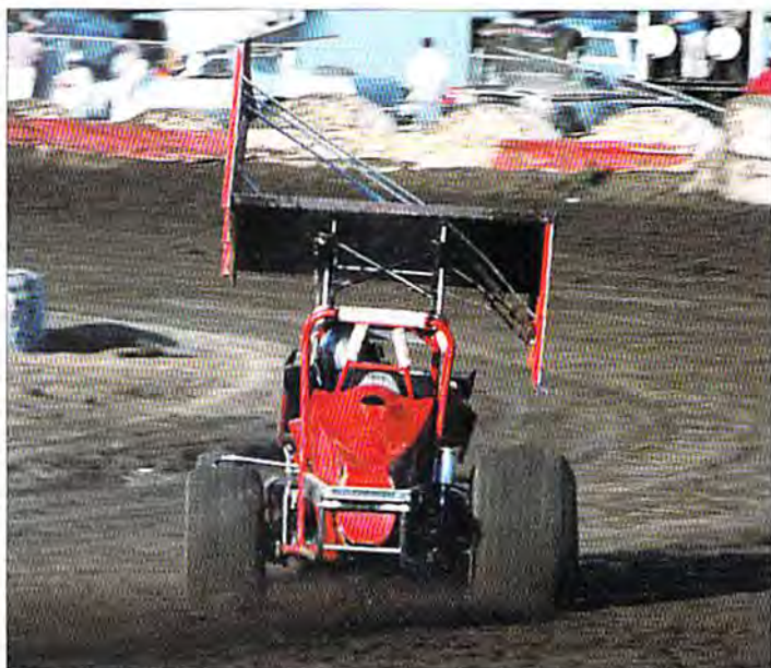
1986: View of the stagger (difference in size of the two tires) on the Ray Terri Super Modified driven by Art McCarthy. Dennis Mattish Photo
